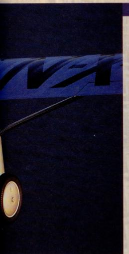
The only way to see ahead in flight was to S-turn while peering out a side window or to boot a rudder pedal. The wing has no dihedral and is so flat that the airplane skids easily toward one side or the other. Lindbergh did not have to worry much about a midair collision in 1927, especially over the Atlantic. Frank Tallman flew a replica for the movie *The Spirit of St. Louis* and said that the airplane "is as blind as a nuclear sub under a polar icepack."
